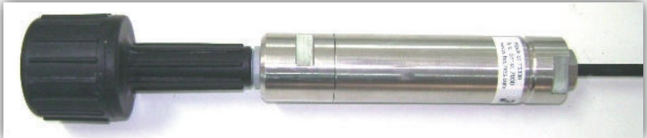
The TECMES sensor, Model TS 330, is a submersible type sensor for the measurement of dissolved oxygen in rivers, reservoirs, treatment plants, etc.
