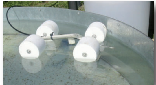
TS 265 sensor with float for evaporation tank
