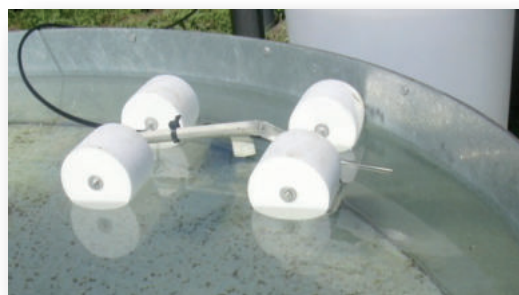
TS 265 sensor with float for evaporation tank
